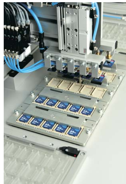
The robot arm picks up the memory cards using suction pads
